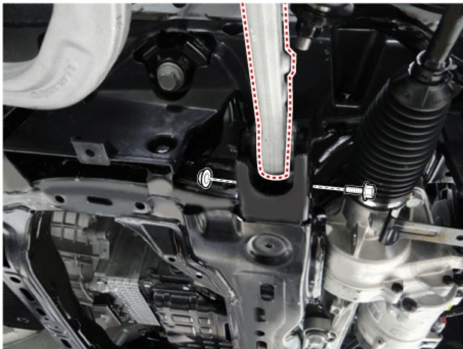
6. Loosen the lateral arm pin (A) and nut (B).
